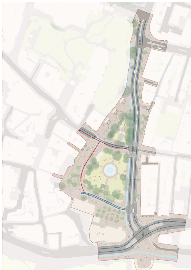
Figures 11 to 13: Preferred Option - Traffic directions. Figure 11 (left) shows the proposed traffic routes and directions for general traffic (dark blue) and buses (red). Figures 12 and 13 (right) show the two northbound and southbound lanes and the central median on eastern side of Steine Gardens from the redesigned A23/259 junction.
